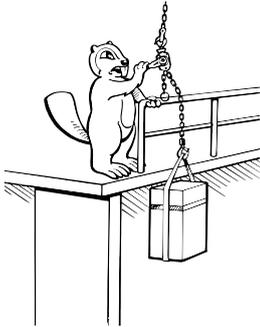
**DO NOT** operate the lever block unless it is rigged to pull in a straight line from hook to hook, and the frame is allowed to freely swivel on the upper hook.
