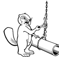
**DO NOT** wrap the load chain around the load and hook onto itself as a choker chain, or bring the load in contact with the lever block.
