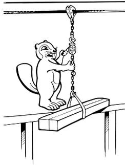
**DO NOT** hold the load chain in a loaded state while operating the lever block as serious injury may occur if the brake did not operate properly.
