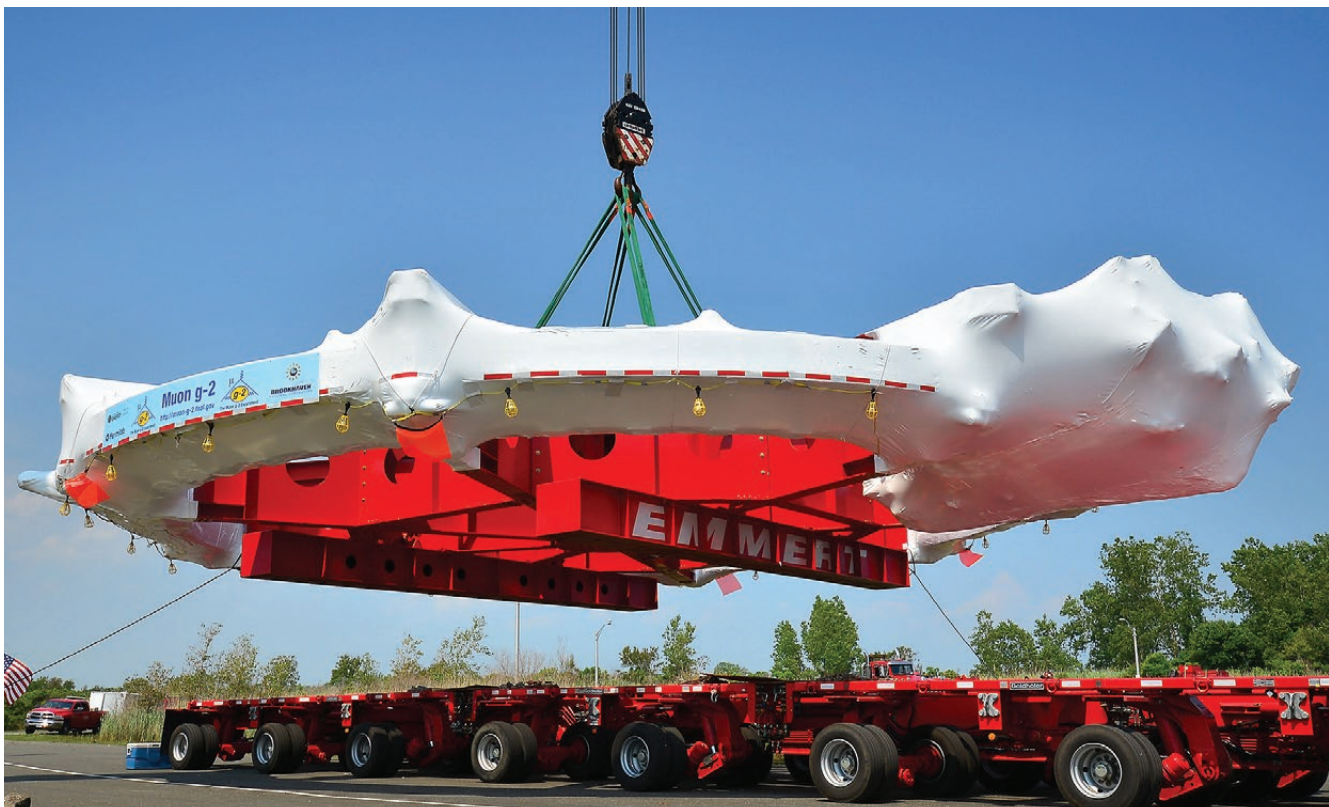
Twin-Path® adjustable bridles self adjust over the centre of gravity.
